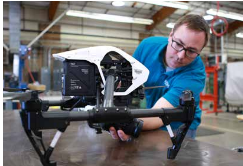
Left photo, Aviation technology instructor Max Moore testing the DJI Inspire 1 Pro drone, which is equipped with a 4K camera and has a maximum speed of 49 miles per hour. Top photo, Moore completes a preflight check before making the Inspire 1 Pro airborne.
