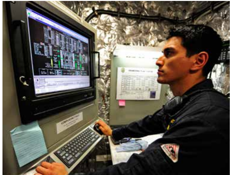
Lt. Julio Alarcon, main propulsion assistant aboard the littoral combat ship USS Independence, uses the engineering control system to transfer fuel between holding tanks in the engineering log room aboard the ship.
